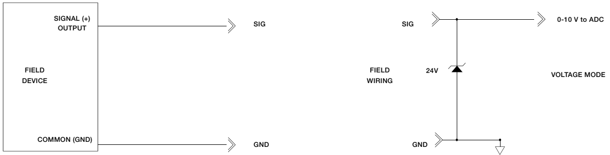
TYPICAL VOLTAGE INPUT FIELDS WIRING
