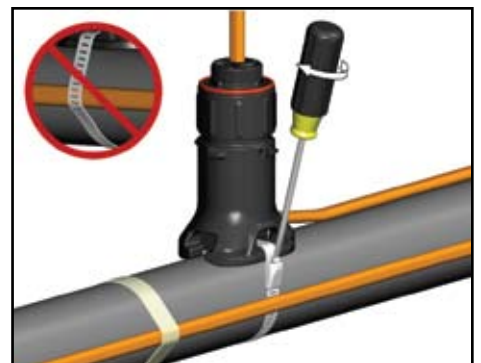
5. Mount expediter to pipe using pipe band. Do not band over cable.
